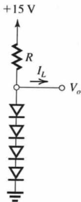
a. In this problem  $\frac{\Delta V_O}{\Delta i_L} = \frac{20 \text{ mV}}{1 \text{ mA}} = 20 \Omega$
