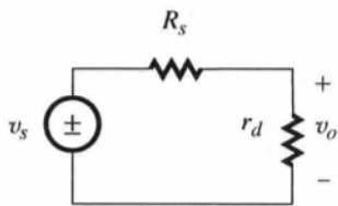
$$v_o = v_s \times \frac{r_d}{r_d + R_s} = v_s \frac{V_T/I}{V_T/I + R_s}$$
